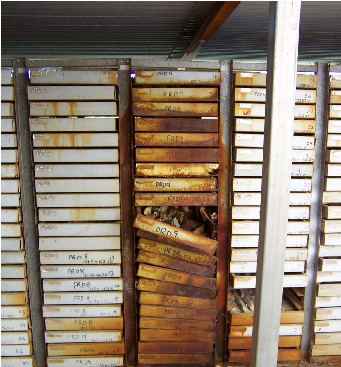
Core samples from the Peak Hill gold mine's sulfide zone left to their own devices (water and air). The DZP's most expensive input will be sulfuric acid, which this deposit may provide, complete with a gold byproduct offset.
